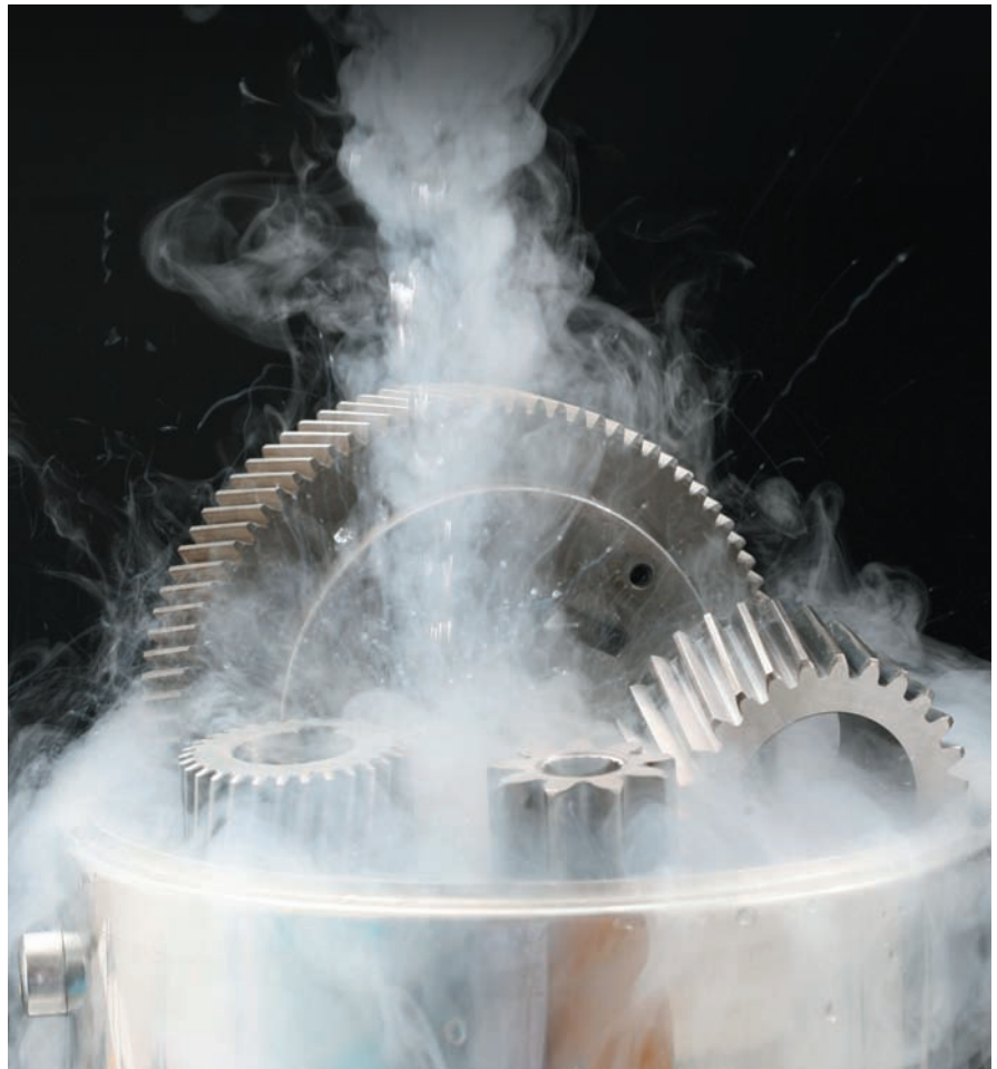
Cold treating gears after quenching.
